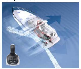
With the joystick the driver can now maneuver the vessel at low speed – with just one hand. The joystick is coupled to a sophisticated and specially developed software that individually commands the electronically controlled engines and underwater units of the system to steer, throttle and shift gears independently, making the boat move in any direction the driver wants – sideways, diagonally, forward, backward or rotate. Visit volvopenta.com to see for yourself!
